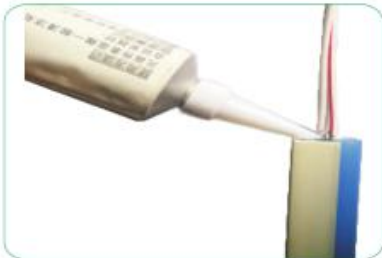
3 Putting some silicone at the location of welding wire
